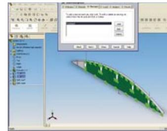
Constraints: The green simulates where the part is held on the milling machine
