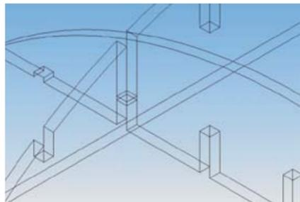
Clock pieces being checked for slot position and interference
