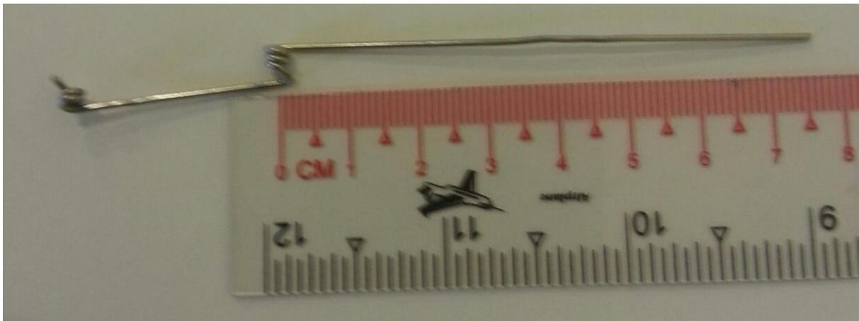
Its currently too long and should be 60mm in length from the coil to the end. Cut it to 60mm.
