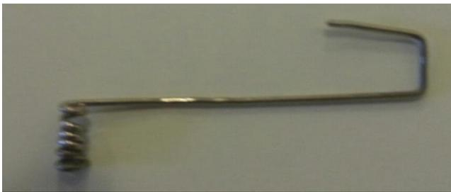
Using pliers, gently straighten the coil (piston) so it is pointing in the correct direction as shown below.
