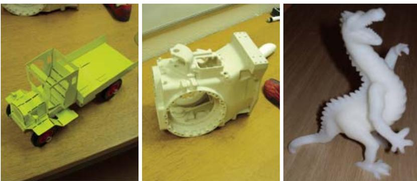
Models above include: sheet metal work for the truck, starch printing for the axle casing and shoe, stereolithography (resin) for the dog lead casing and FDM for the dinosaur.
